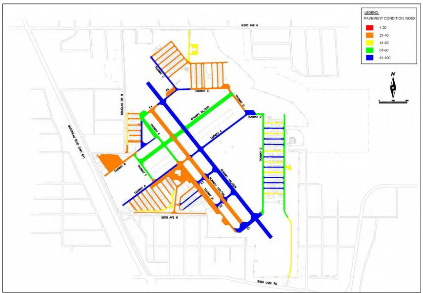
Figure 2-2: Crystal Airport Pavement Condition Index (2014 PCI)
